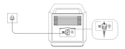
**Note:** When the AC input is connected to the mains, if you do not need to use the AC output, please turn off the AC output switch, otherwise it will reduce the AC charging power.
